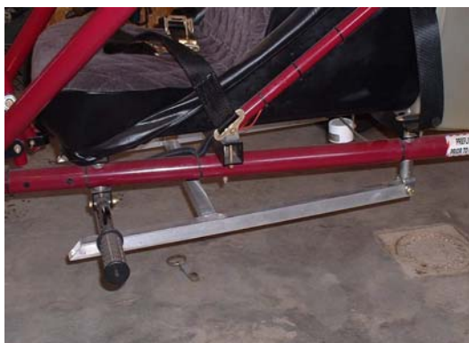
The Suke-Stopper in the "UP" position. A clevis pin keeps it from coming down inadvertently.
