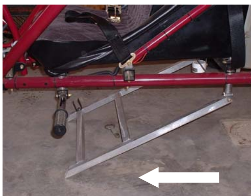
The Suke-Stopper in the deployed position. Forward thrust would drive the device into the ground to keep the plane from moving forward.
